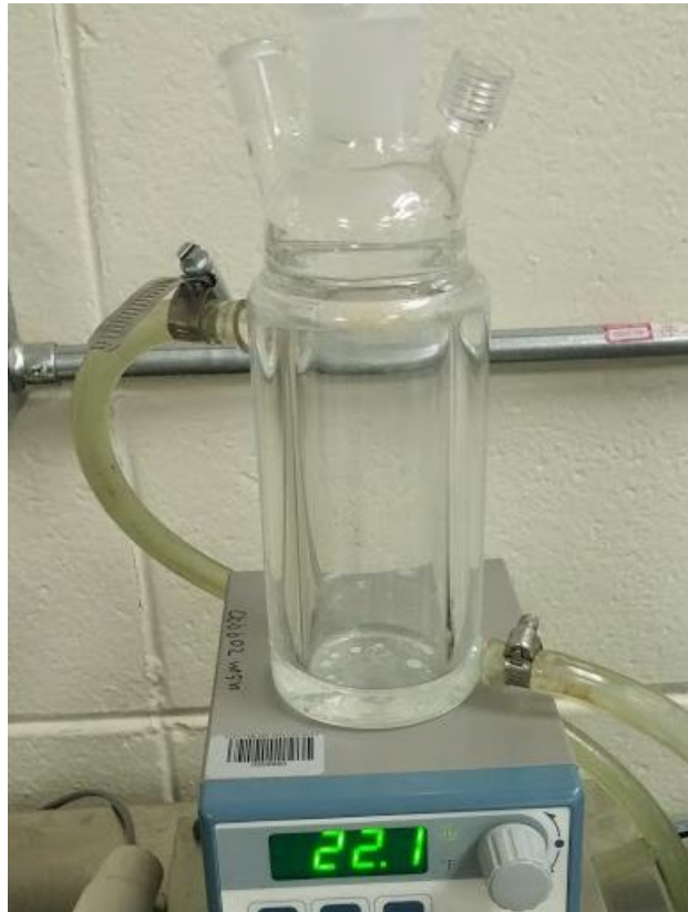
Figure 5 – Temperature controlled 200 mL jacketed flask used as test chamber.
